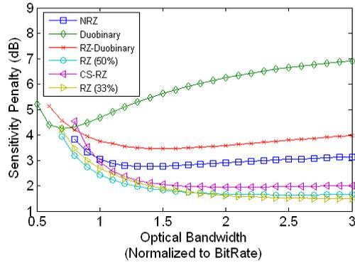
**Fig. 3.3. QL sensitivity penalty to achieve  $\text{BER}=10^{-9}$  for fixed electrical bandwidth.  $B_e = 0.7 \cdot R$  for NRZ and RZ formats and  $B_e = 1 \cdot R$  for DB formats. With the exception of DB, performance is fairly flat beyond  $B_o = 1.5 \cdot R$ .**
