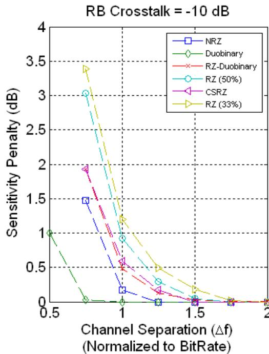
**Fig. 3.13. Excess penalty for using ASE-limited optical receiver as a function of incoherent RB level. The penalty for using an ASE-optimized receiver is large for tight channel packing density.**
