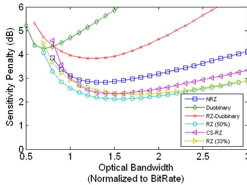
**Fig. 3.11. QL sensitivity penalty to achieve  $BER=10^{-9}$  in the presence of 20 dB of RB crosstalk for fixed electrical bandwidth.  $B_e = 0.7 \cdot R$  for NRZ and RZ formats and  $B_e = 1 \cdot R$  for DB formats.**
