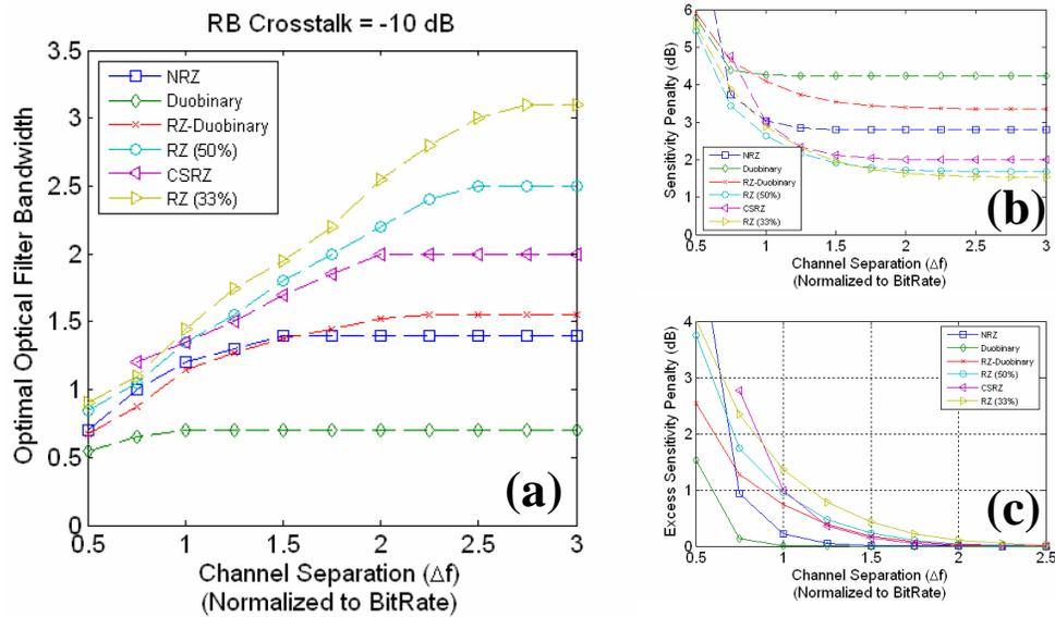
**Fig. 3.12. QL performance under optimal receiver condition as a function of channel separation between signal and RB. (a) Optimal optical filter bandwidth. (b) Absolute QL penalty. (b) Excess QL penalty relative to case without RB crosstalk.**
