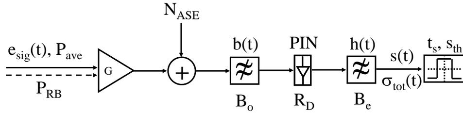
**Fig. 3.1. Schematic diagram of the preamplified receiver model. Additional mathematical descriptions of the various parameters can be found in Chapter 2. In this study,  $G = 27$  dB and  $NF = 3$  dB (ideal amplification).**
