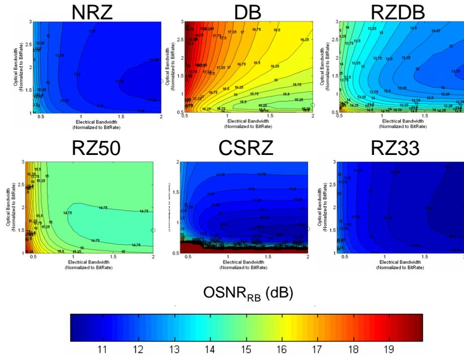
**Fig. 3.4. Coherent RB-limited contour plots of constant QL to attain BER=10<sup>-9</sup>. Optimal B<sub>o</sub>/B<sub>e</sub> combinations designated by circles. Values quoted in absolute OSNR<sub>RB</sub> (dB) required to maintain BER = 10<sup>-9</sup>.**
