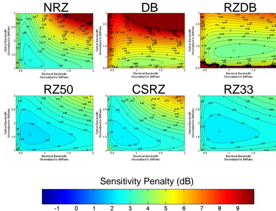
**Fig. 3.10.** QL sensitivity penalty to achieve  $\text{BER}=10^{-9}$  in the presence of 20 dB of RB crosstalk for fixed electrical bandwidth.  $B_e = 0.7 \cdot R$  for NRZ and RZ formats and  $B_e = 1 \cdot R$  for DB formats.
