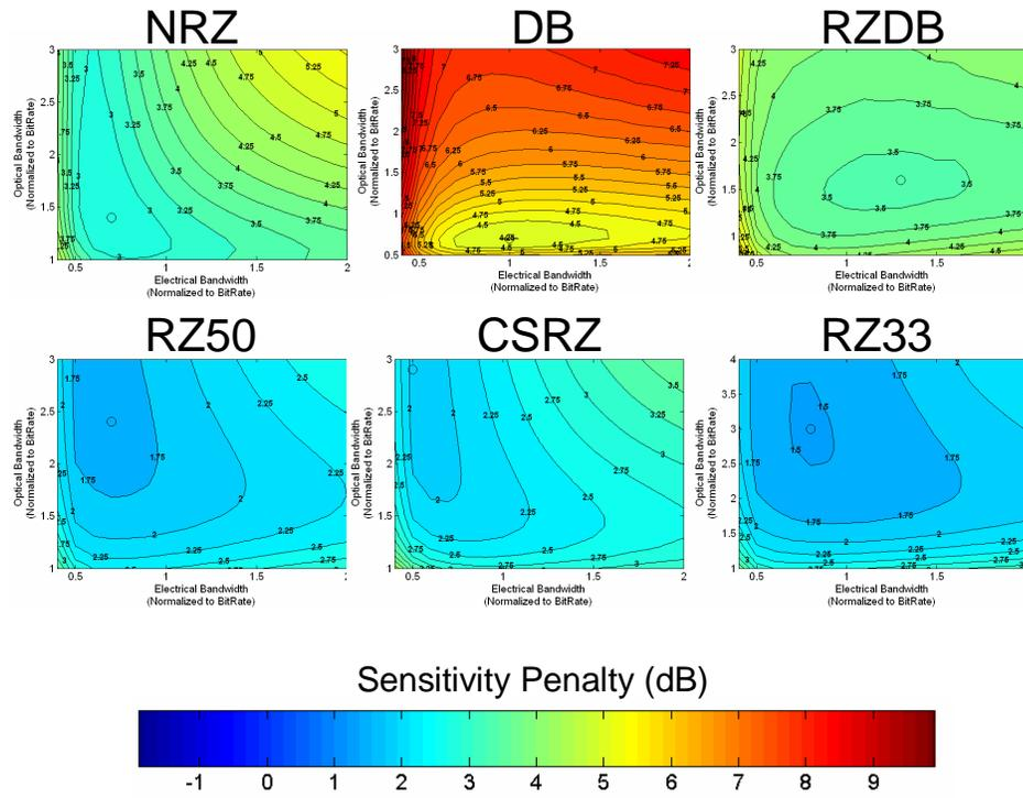
**Fig. 3.2. ASE-limited contour plots of constant QL to attain  $BER=10^{-9}$ . Optimal  $B_o/B_e$  combinations designated by circles.**
