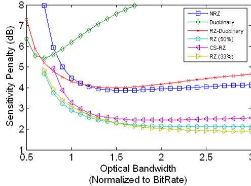
**Fig. 3.7. QL sensitivity penalty to achieve  $BER=10^{-9}$  in the presence of 20 dB of RB crosstalk for fixed electrical bandwidth.  $B_e = 0.7 \cdot R$  for NRZ and RZ formats and  $B_e = 1 \cdot R$  for DB formats.**
