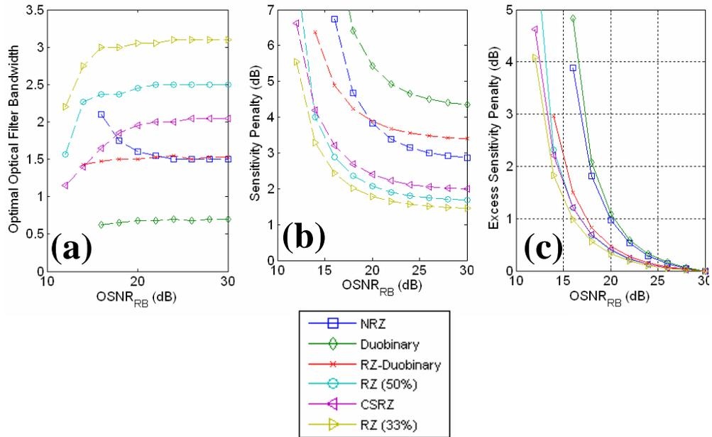
**Fig. 3.8.** QL performance under optimal receiver condition as a function of coherent RB level. (a) Optimal optical filter bandwidth. (b) Absolute QL penalty. (b) Excess QL penalty relative to case without RB crosstalk.
