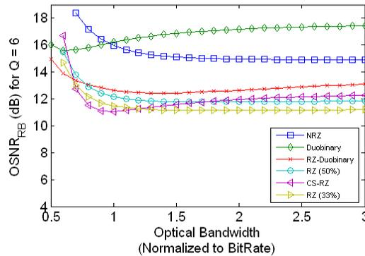
**Fig. 3.5. Required OSNR<sub>RB</sub> to achieve BER=10<sup>-9</sup> for fixed electrical bandwidth. B<sub>e</sub> = 0.7\*R for NRZ and RZ formats and B<sub>e</sub> = 1\*R for DB formats. With the exception of DB, performance is fairly flat beyond B<sub>o</sub> = 1.5\*R.**
