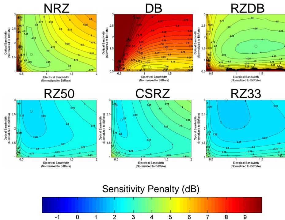
**Fig. 3.6.** ASE-limited contour plots of constant QL to attain  $\text{BER}=10^{-9}$  in the presence of 20 dB of RB crosstalk (i.e.  $\text{OSNR}_{\text{RB}} = 20$  dB into preamplifier). Optimal  $B_o/B_e$  combinations designated by circles.
