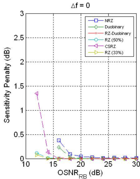
**Fig. 3.9.** Excess penalty for using ASE-limited optical receiver as a function of coherent RB level. The penalty for using an ASE-optimized receiver is minimal.
