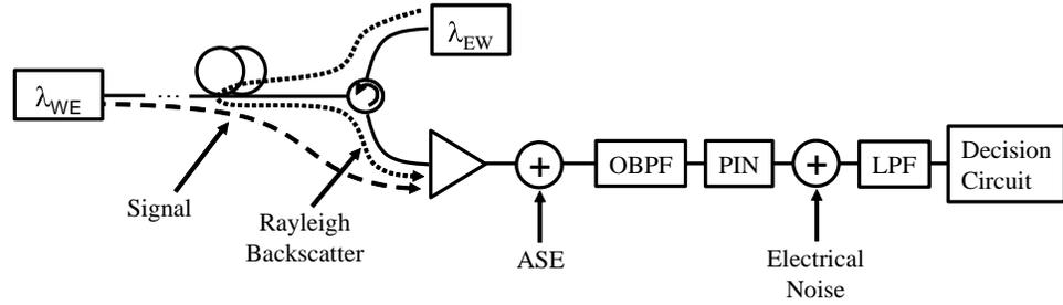
**Fig. 2.1. Conceptual schematic of the system under investigation. The W-E signal is detected in the presence of RB noise generated from the E-W signal. Three types of noise are always present in the studied system: ASE, RB and electrical noise from the detection circuitry.**
