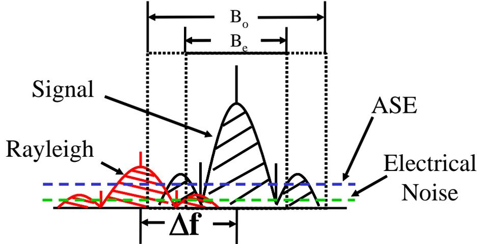
**Fig. 2.2.** Frequency domain illustration of the detection process of the W-E signal from Fig. 2.1. RB caused by the E-W channel is colored while ASE and electrical noise are white. The detected signal lies centered within the electrical bandwidth,  $B_e$ , and the optical bandwidth,  $B_o$ .
