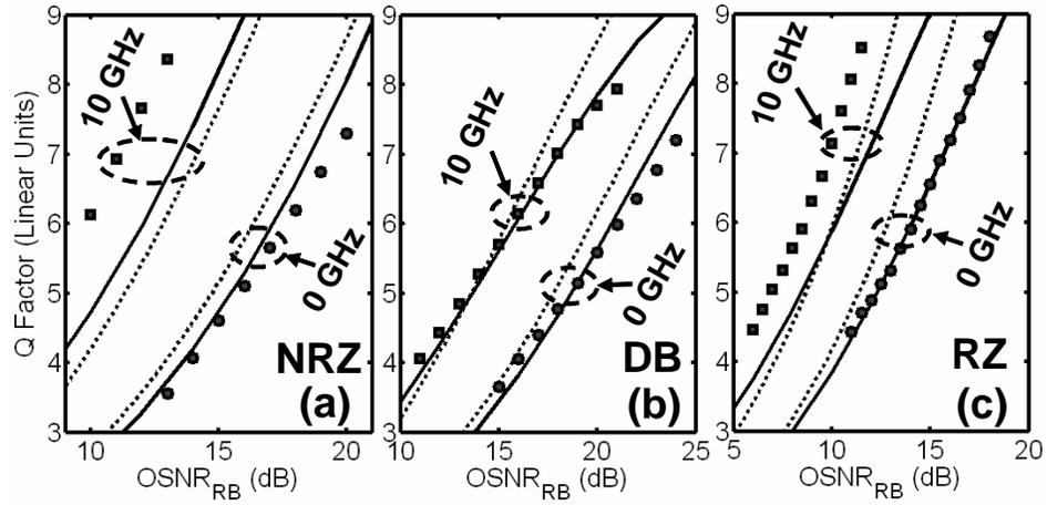
**Fig. 2.11. Results showing copolarized RB impact on Q-factor for  $\Delta f = 0$  and  $\Delta f = 10$  GHz for (a) NRZ (b) DB (c) RZ. Markers—measured points. Solid curve—exact PSD solution, dashed—approximate PSD solution.**
