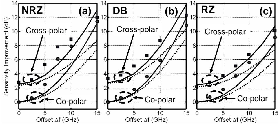
**Fig. 2.12. Theoretical and experimental results showing enhanced RB sensitivity for larger offset,  $\Delta f$ , for (a) NRZ (b) DB (c) RZ. Markers—measured points. Solid curve—numerical solution, dashed—analytic solution.**
