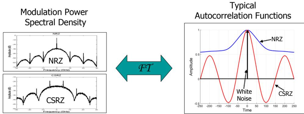
**Fig. 2.3. Illustration showing the Fourier Transform relationship between the modulation PSD and the respective ACF. Figures are generated using the numerical model code.**
