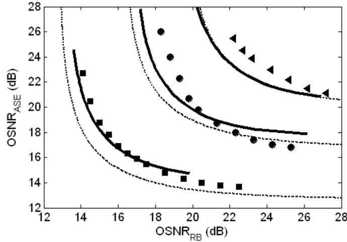
**Fig. 2.10. Contour plots of constant  $Q = 6$  for combination of ASE and coherent RB. Dashed line—analytic model. Solid line—numerical model. Marks—experimentally measured data.**
