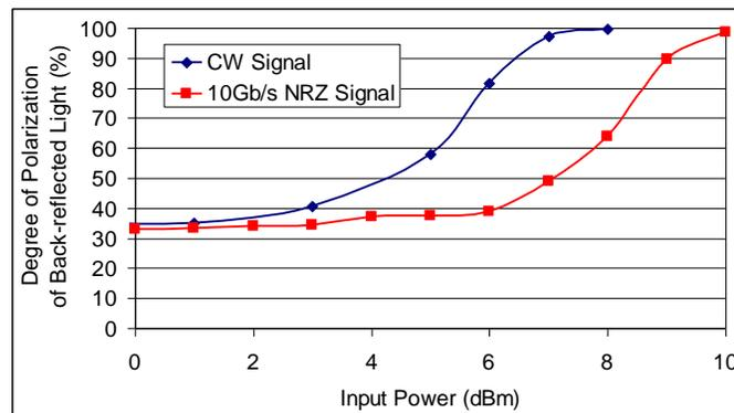
**Fig. 2.6. Degree of polarization of the backreflected light versus input power. In the Rayleigh region the DOP is 33% [14]. As launch power increases, DOP increases towards 100% since SBS light is polarized [29].**
