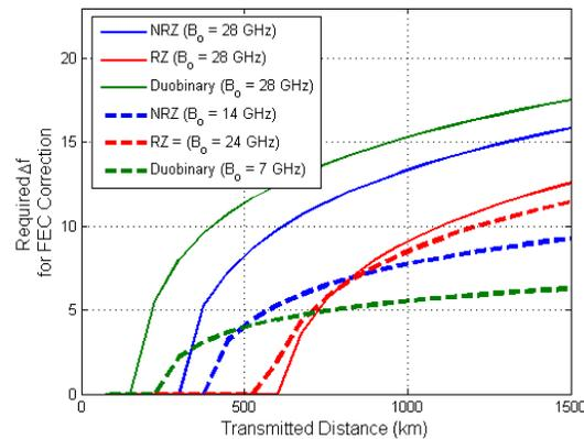
**Fig. 2.13. Required channel spacing in an IB topology to achieve errorless signaling using FEC. Solid lines correspond to non-ideal demux bandwidths (28 GHz). Dashed lines correspond to “ideal” ASE optimized demux bandwidths. Beyond 700 km, DB has superior performance in terms of SE.**
