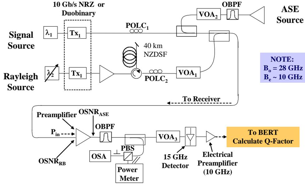
**Fig. 2.8. Experimental setup. Polarization Controller—POLC. Variable optical attenuator—VOA. Polarization beam splitter—PBS. Bit error rate tester—BERT. Optical spectrum analyzer—OSA.**
