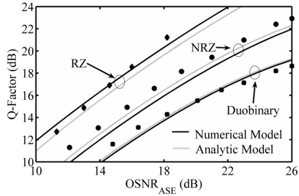
**Fig. 2.9. Comparison of theory and experiment for ASE dominated performance.**
