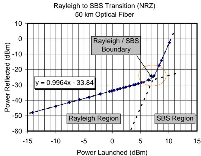
**Fig. 2.5. Backreflected power versus launched power into single mode fiber. In the Rayleigh region, the reflected power increases dB for dB with launched power. At the onset of SBS, backreflected power begins to increase rapidly after the Rayleigh/SBS boundary.**
