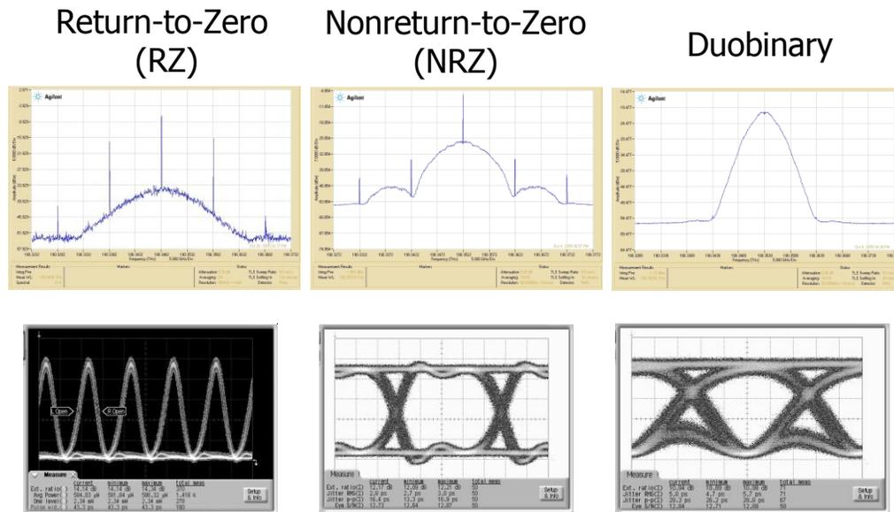
**Fig. 2.4. Experimental modulation spectra and eye diagrams for 10 Gb/s RZ, NRZ and DB.**
