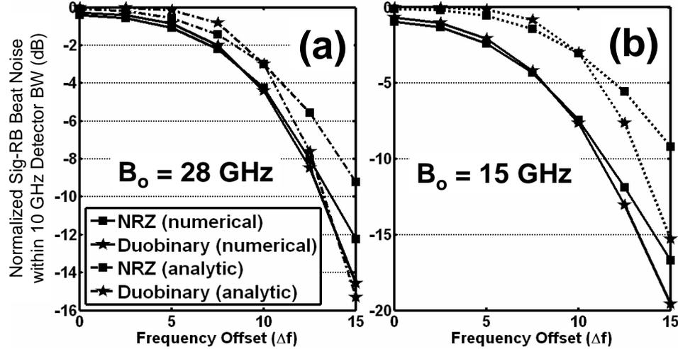
**Fig. 2.14.** Normalized Signal-RB beat noise within a 10 GHz detector bandwidth for exact and approximate PSDs. (a)  $B_o = 28$  GHz, (b)  $B_o = 15$  GHz. Discrepancy between analytic and numerical models for DB is smaller and for NRZ.
