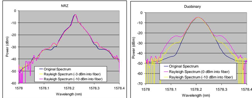
**Fig. 2.7. RB spectrums for NRZ and DB. Stokes shifts of +/-11 GHz visible due to spontaneous Brillouin scattering. RB PSD is proportional to the launched PSD.**
