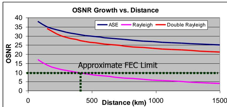
**Fig. 1.4. Calculation of ASE, RB and DRB in example link from Fig. 1.3. RB noise severely limits performance when counter-propagating channels use the same wavelength.**
