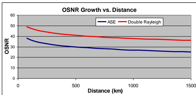
**Fig. 1.2. Growth of ASE and DRB in the unidirectional system in Fig. 1.1. ASE limits performance but can be maintained below significant levels for thousands of km with proper link design. Values assumed in the calculation:  $L = 75$  km, fiber loss = 0.2 dB/km,  $G = 15$  dB, amplifier noise figure (NF) = 5 dB, launched power = 1 mW (0 dBm), Rayleigh scattering coefficient per/span = -32 dB.**
