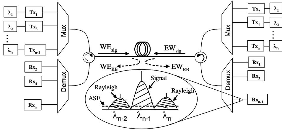
**Fig. 1.5. Interleaved Bidirectional System. Duplex communication is possible by transmitting unidirectionally on alternating channel. RB crosstalk from adjacent channels is mitigated by filtering in the demultiplexer (demux).**
