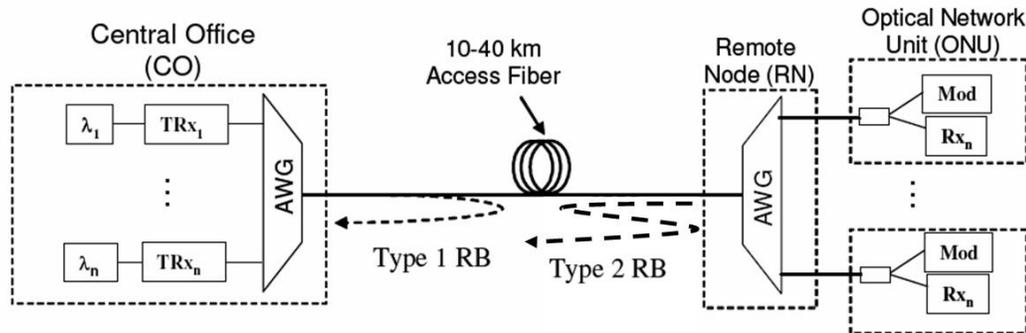
**Fig. 1.6. CLS-PON Topology.** Placing the light source at the CO allows for flexible wavelength allocation to the customers. The ONU must only provide modulation and detection. RB limits systems margin and devices caused by both the downstream (Type 1) and upstream (Type 2) launched light.
