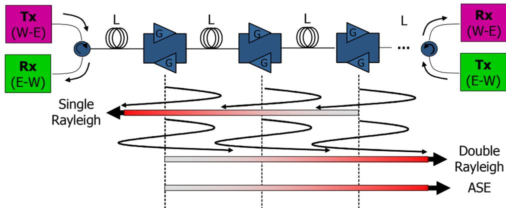
**Fig. 1.3. Example of a bidirectional fiber link with both east-west (E-W) and west-east (W-E) communication. Isolators not feasible since information travels in both directions on the same wavelength.**
