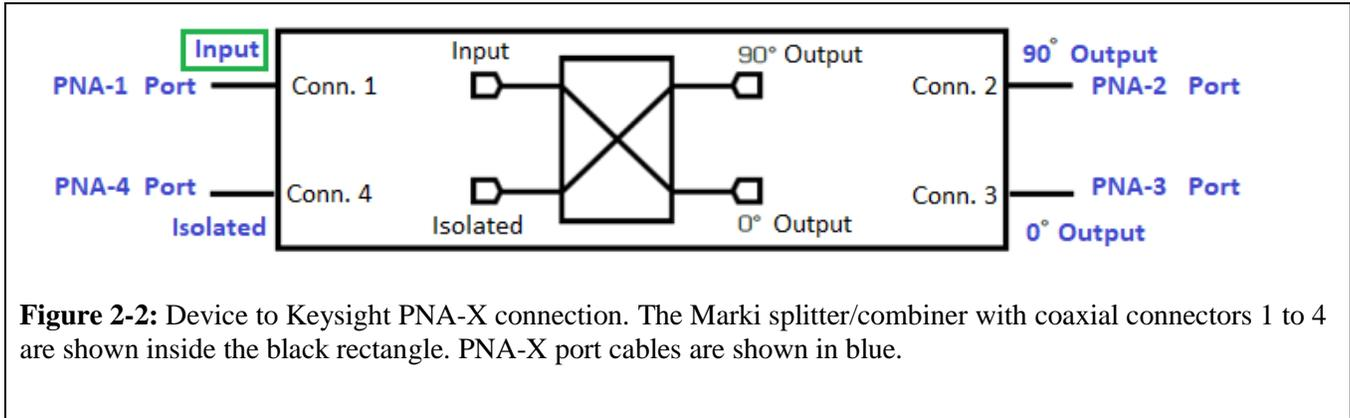
**Figure 2-2:** Device to Keysight PNA-X connection. The Marki splitter/combiner with coaxial connectors 1 to 4 are shown inside the black rectangle. PNA-X port cables are shown in blue.
