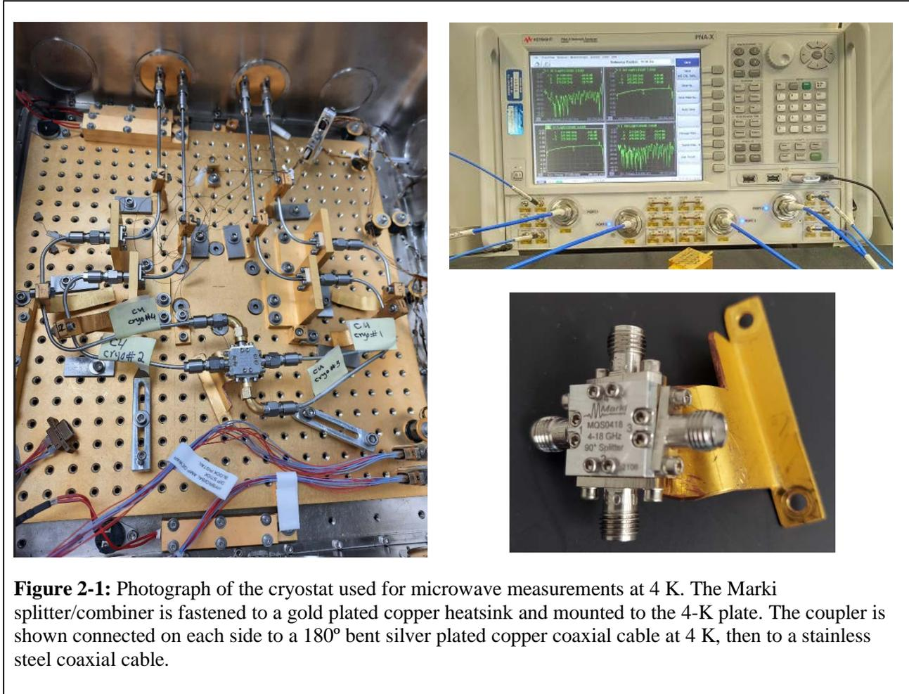
**Figure 2-1:** Photograph of the cryostat used for microwave measurements at 4 K. The Marki splitter/combiner is fastened to a gold plated copper heatsink and mounted to the 4-K plate. The coupler is shown connected on each side to a 180° bent silver plated copper coaxial cable at 4 K, then to a stainless steel coaxial cable.
