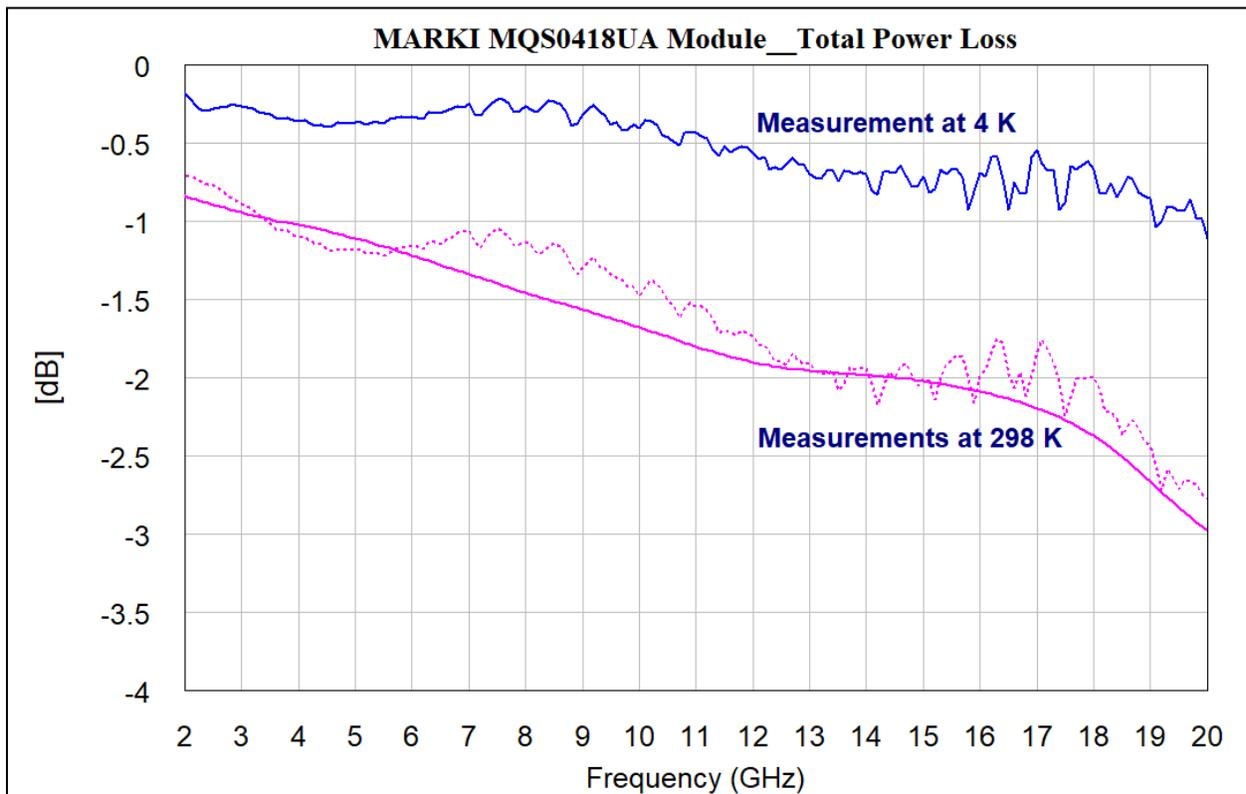
**Figure 3-3:** Comparison of warm ( $T = 298 \text{ }^\circ\text{K}$ , Magenta traces) and cold ( $T = 4 \text{ }^\circ\text{K}$ , Blue trace) total power loss of the splitter/combiner. The solid magenta trace corresponds to measurement directly on the PNA-X, and the dotted magenta trace corresponds to the in-cryostat warm measurement de-embedded with the Keysight AFR software. The difference between the warm measurements are an indication of the error in the cold measurements.
