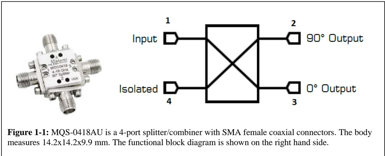
**Figure 1-1:** MQS-0418AU is a 4-port splitter/combiner with SMA female coaxial connectors. The body measures 14.2x14.2x9.9 mm. The functional block diagram is shown on the right hand side.
