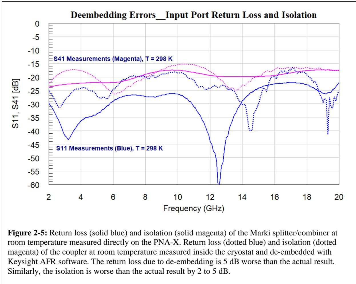
**Figure 2-5:** Return loss (solid blue) and isolation (solid magenta) of the Marki splitter/combiner at room temperature measured directly on the PNA-X. Return loss (dotted blue) and isolation (dotted magenta) of the coupler at room temperature measured inside the cryostat and de-embedded with Keysight AFR software. The return loss due to de-embedding is 5 dB worse than the actual result. Similarly, the isolation is worse than the actual result by 2 to 5 dB.
