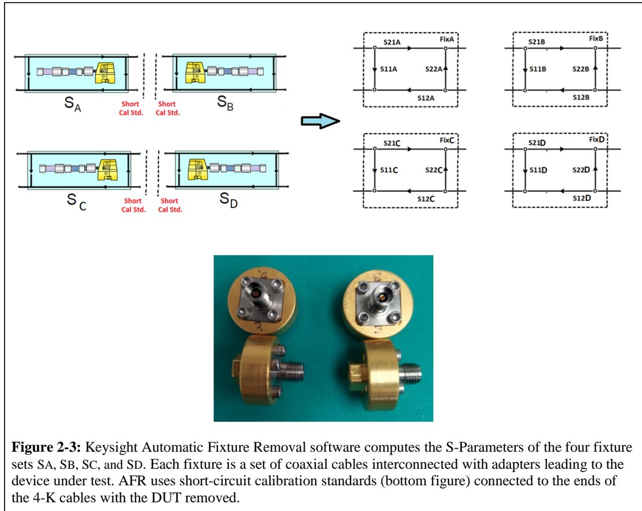
**Figure 2-3:** Keysight Automatic Fixture Removal software computes the S-Parameters of the four fixture sets SA, SB, SC, and SD. Each fixture is a set of coaxial cables interconnected with adapters leading to the device under test. AFR uses short-circuit calibration standards (bottom figure) connected to the ends of the 4-K cables with the DUT removed.
