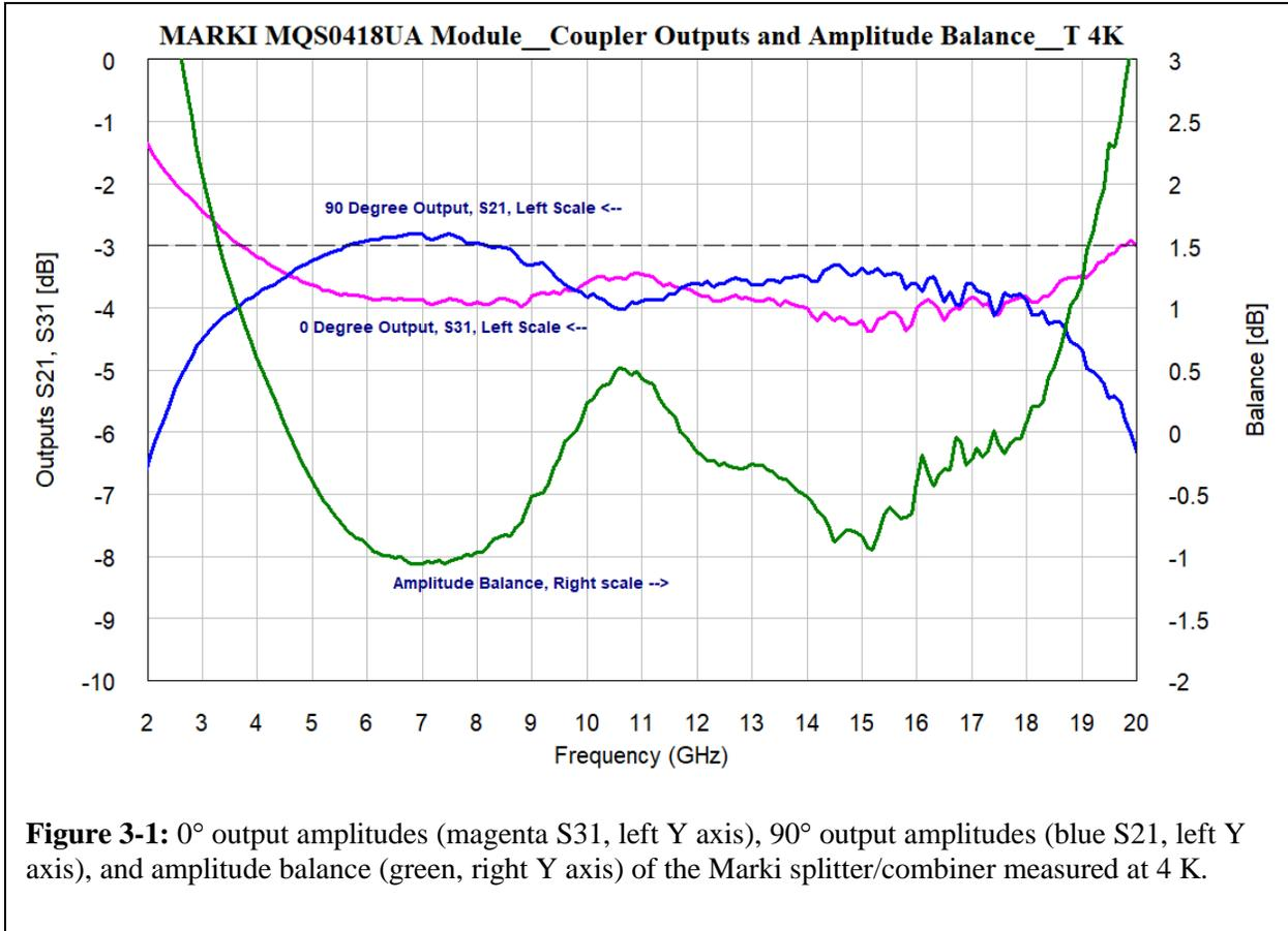
**Figure 3-1:** 0° output amplitudes (magenta S31, left Y axis), 90° output amplitudes (blue S21, left Y axis), and amplitude balance (green, right Y axis) of the Marki splitter/combiner measured at 4 K.
