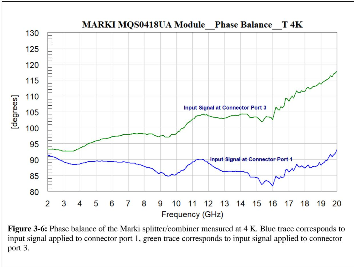
**Figure 3-6:** Phase balance of the Marki splitter/combiner measured at 4 K. Blue trace corresponds to input signal applied to connector port 1, green trace corresponds to input signal applied to connector port 3.
