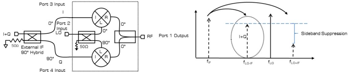
A single sideband mixer is a mixer which suppress the up converted image frequency from the RF output. Single sideband mixers are constructed using an external quadrature hybrid attached to the I and Q (i.e., IF) input ports. Using an external IF quadrature hybrid, one can select whether the upper sideband of the lower sideband signal is suppressed with respect to the LO signal.
