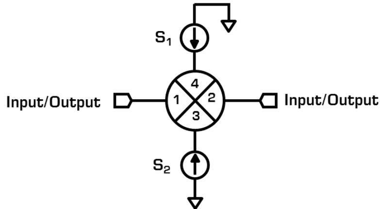
A vector modulator is a device that can modulate an input signal's amplitude and phase. Similar to using a double balanced mixer as a phase modulator or phase shifter, an IQ mixer can be used as a vector modulator. An IQ mixer can be used as a vector modulator by inputting DC current into both the I and Q ports.
