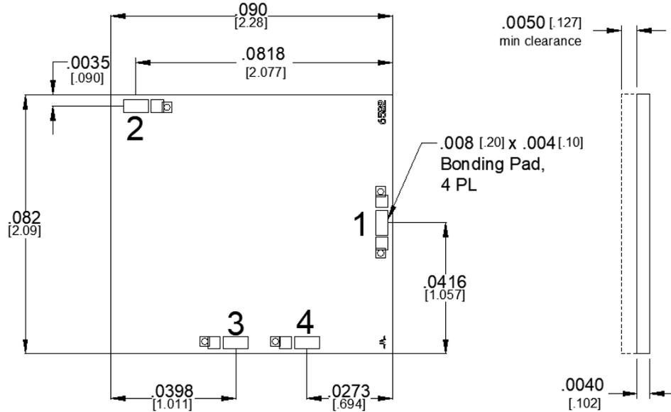
1. CH substrate is 0.004 in thick GaAs.
