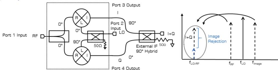
An image reject mixer is a mixer which rejects the down converted image frequency from the IF output. Image reject mixers are constructed using an external quadrature hybrid attached to the I and Q (i.e., IF) output ports. Using the external IF quadrature hybrid, one can select the whether the upper sideband or lower sideband signal is suppressed with respect to the LO signal.
