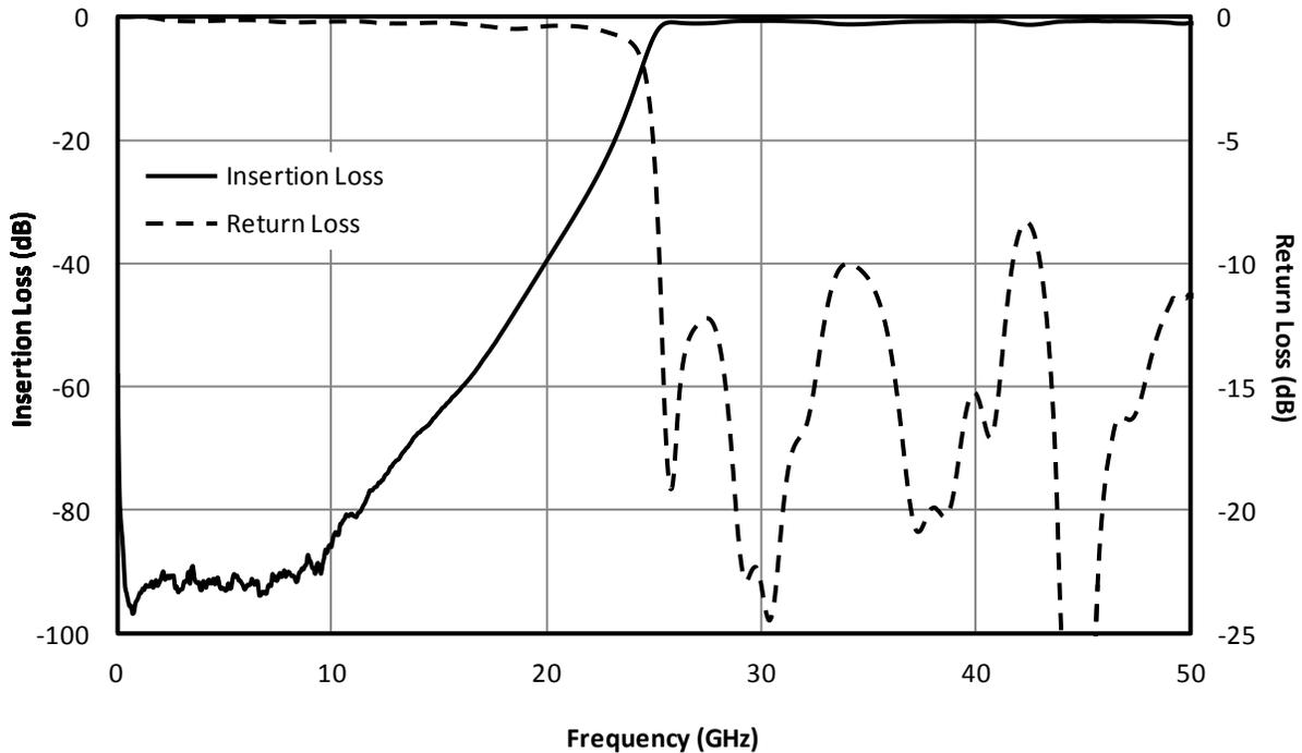
Fig. 1. Magnitude response for a typical FH-2600 Filter.
