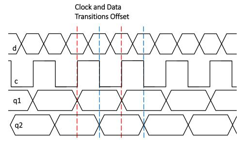
The duty cycle of the clock should be between 45% and 55%. The duty cycle can be adjusted by biasing the dcp and dcn pins between 0 and -3.3 V. If duty cycle adjustment is not required these pins may be left unconnected.
