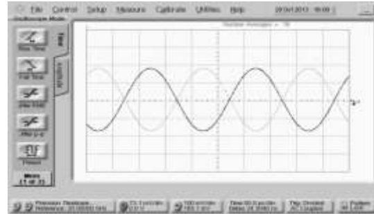
Fig. 6. Oscilloscope measurements with 5 GHz sine wave input. Excellent amplitude and phase balance are apparent. Note that BAL-0106 is not suitable for baseband data, as any data input will be high pass filtered, particularly on the inverted side.
