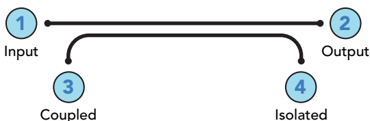
Figure 1: Schematic diagram of a directional coupler.
