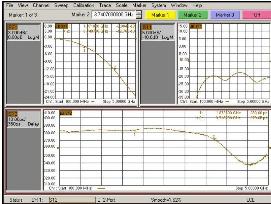
Fig. 1. Magnitude Response (Top) and Group Delay Response (Bottom) for a typical 1.87 GHz Wavefade™ measured at an Aperture of 80 MHz.
