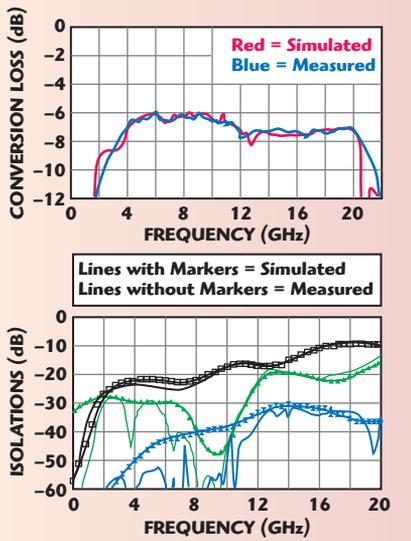
▲ Fig. 3 Microlithic mixer simulated and measured performance.
