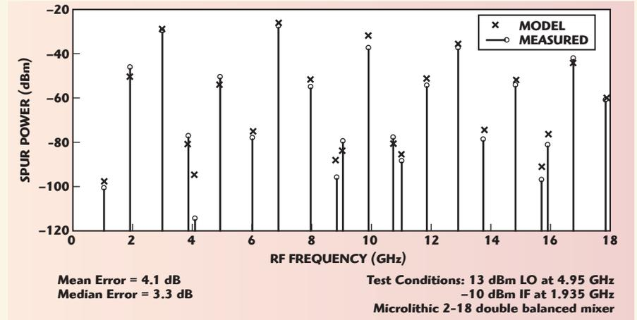
▲ Fig. 4 Measured spur level vs. microlithic model (MWO).
