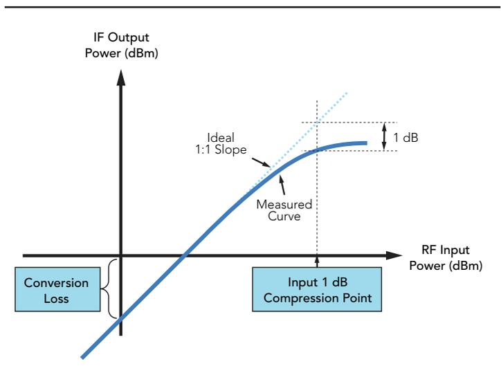
Figure 9: Graphical representation of 1 dB compression point.
