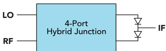
**Figure 5: Single balanced mixer with 4-port hybrid junction.**
