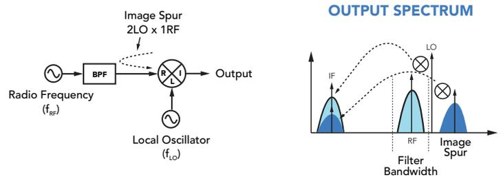
**Figure 10: Schematic diagram (left) showing backreflected 2LO x 1RF spur from reactive bandpass filter (BPF). Output spectrum (right) showing desired IF and downconverted image spur overlapping in frequency.**
