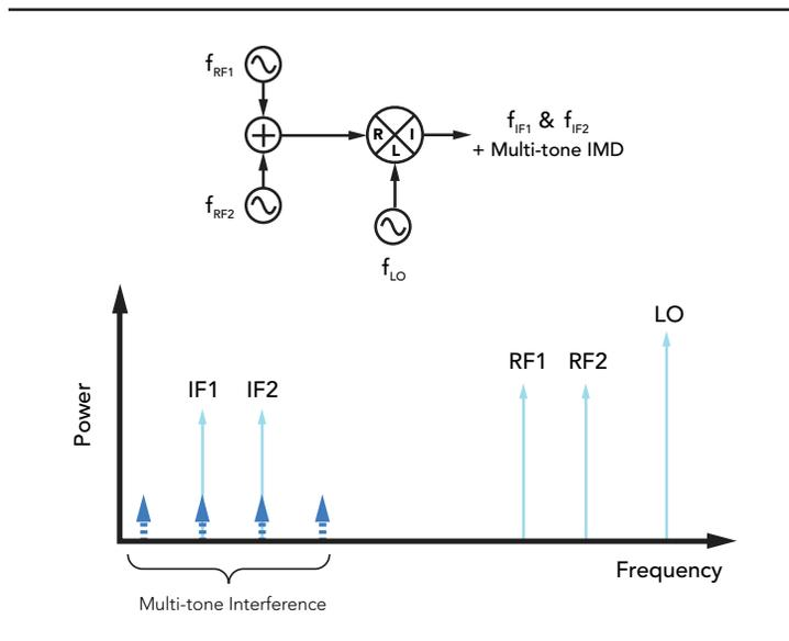
**Figure 12: Illustration of multi-tone IMD created by two closely spaced RF signals. Generated IMD tones overlap with desired IF<sub>1</sub> and IF<sub>2</sub> signals.**
