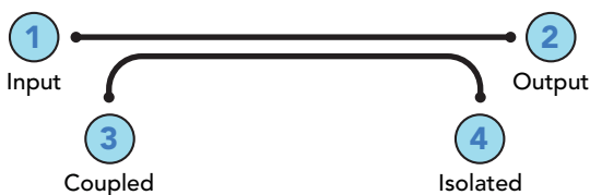
Figure 1: Schematic diagram of a directional coupler.
